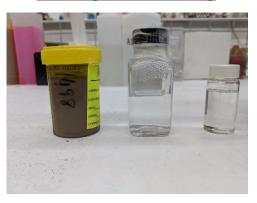
Drilling mud traced at various depths to determine invasion of the traced coring fluid and estimate the final core water saturation level.
