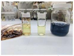
Polymer traced with one of our IsoTECH formulations to provide producer with information if produced polymer was current or past application.
